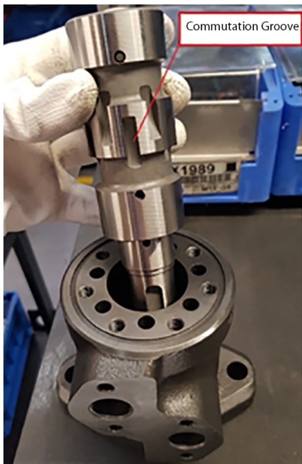
Figure 7: Correct positioning of shaft (offset ports):
