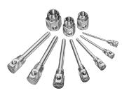
These tools are required for assembling 069 'D' Series hose ends in sizes 4 through 12 to prevent cutting the hose inner tube. Size 16 through 32 mandrels are used as a holding device when assembling 069 'D' Series swivel ends. Mandrels can be ordered individually.
