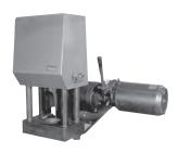
The T-400-PH conversion kit is designed to allow the use of standard Weatherhead Coll-O-Crimp tooling, hose, and hose ends in the Parker 80c crimper. Everything is included to convert the crimper to accept Weatherhead tooling. This kit gives the crimper capacity to crimp up to and including 1-1/4" I.D. 2-wire hose factory-type hose assemblies.
