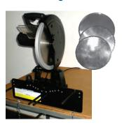
This cutting machine easily handles all 1 and 2 braided wire hose through 4" I.D., up to 2" I.D. 4-spiral and up to 1-1/2" I.D. 6 multi-spiral reinforced hose. That makes this machine ideal for cutting most hydraulic and pneumatic hoses as well as a variety of industrial fluid transfer hoses. The T-71 uses a 14" cutting blade, T-1070, for cutting all 1 & 2 wire braid and through 2" 4 spiral hose. The scalloped toothed blade T-1071, is for cutting industrial
