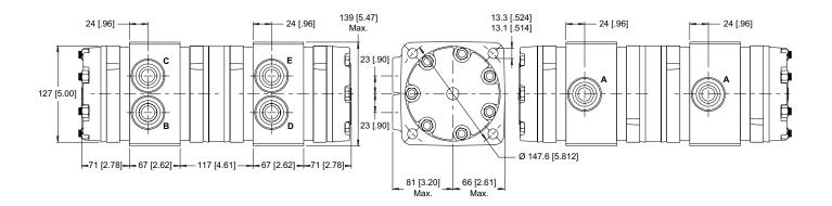
▶ The flow rate range is 19-189 lpm [5-50 gpm] and has a weight of 34.9 kg [77 lb]. 950 Series weights vary ± 0.9 kg [2 lb] based on model configuration. By changing the first A in the model code to a Z, the unit will be unpainted instead of the standard black paint. Ports A, B, C, D & E are 1 1/16-12 UN.
