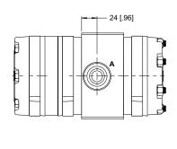
► The flow rate range is 15-141 lpm [4-40 gpm] and has a weight of 24.1 kg [53 lb]. 950 Series weights vary ± 0.9 kg [2 lb] based on model configuration. By changing the first A in the model code to a Z, the unit will be unpainted instead of the standard black paint. Ports A, B & C are 1 1/16-12 UN. Port F is 7/18-14 UNF.
